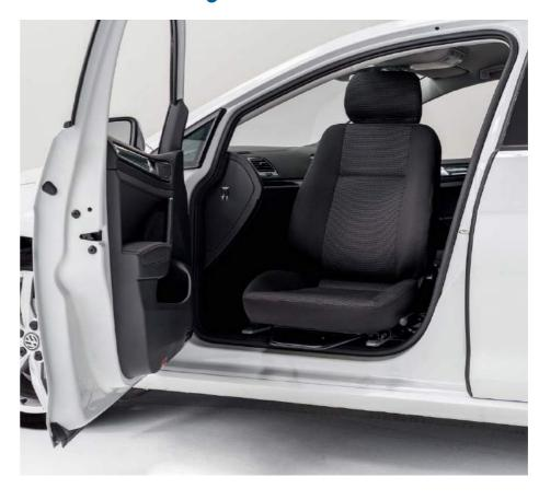
Swivels the car seat outside the vehicle for easy access.
