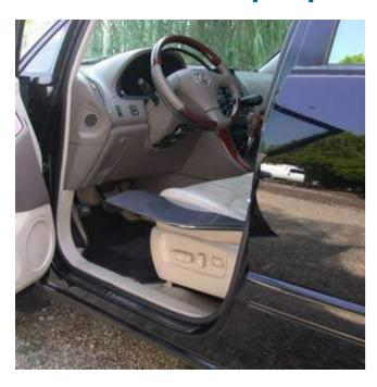
The Manual Tip Up Plate enables users to transfer onto a car seat with ease.
