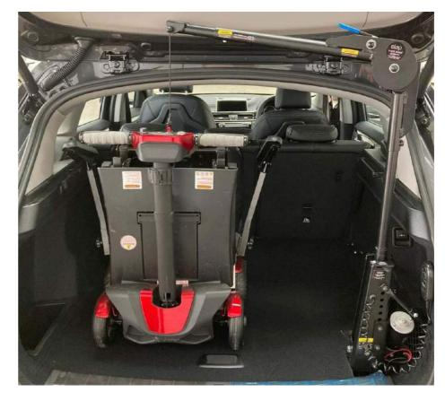
The Elap V40X Wheelchair and Scooter Hoist allows users to move a wheelchair/scooter in and out of a vehicle via the touch of a button.
