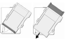
By reversing the seat halfway through the swivel process valuable space has been created for users legs and feet. This is one of the key features that now makes it possible to choose vehicles that previously have been considered too small and narrow to install.
